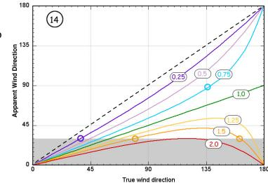
As the boat's speed increases with respect to the wind (larger values of the ratio) this effect becomes more pronounced.
