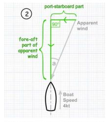
**Step 1.** The boat's motion only changes the fore-aft part of the wind. So we first split the apparent wind into fore-aft and port-starboard components by drawing a scale diagram as in **figure 2**.
