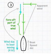
**Step 2.** Now take away the effect of the boat's movement by shortening the fore-aft part of the apparent wind by an amount representing the speed of the boat (**Figure 3**). This gives us the fore-aft component of the true wind.
