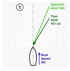
The result is summarised in **Figure 5**. When the wind is from ahead, the true wind is further aft and less in magnitude compared to the apparent wind.
