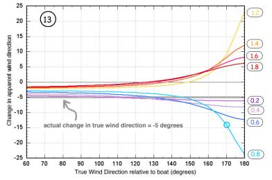
changes by nearly  $15^{\circ}$  and goes even more to starboard. The various curves show that this magnification of the change in wind direction is most pronounced when the true wind direction is within  $20^{\circ}$  of the stern, and when the boat's speed is close to the true wind speed.
