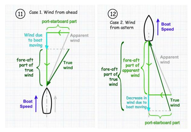
The difference in wind direction between the apparent wind and the true wind is due to the speed of the boat. It therefore follows that the faster the boat is travelling compared to the wind, the closer the apparent wind will be to the bow.
