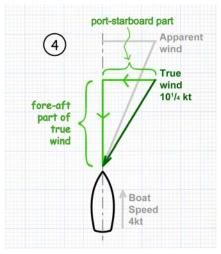
**Step 3. Figure 4** shows how to recombine the foreaft and port-starboard components to find the speed and direction of the true wind.
